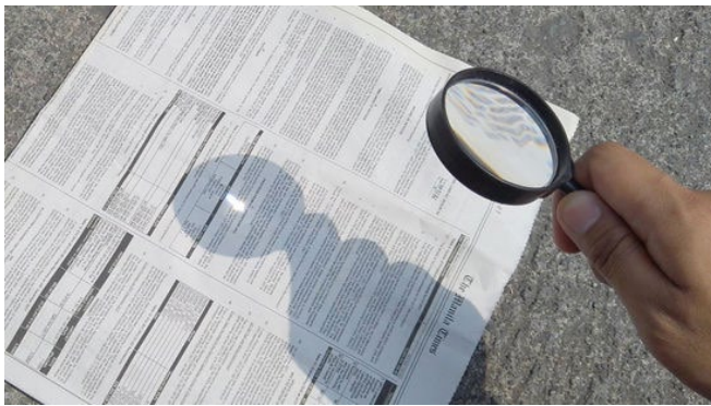
Burning Paper using Convex Lens
